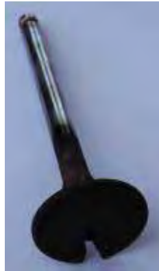
Fig. 2. Exhaust valve out of order
