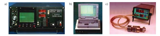
*Fig. 1. Portable pressure analyzers developed and applied in Poland: a) – ACS-4 analyzer, b) – MA2000 analyzer, c) – UNITEST 203 analyzer*
