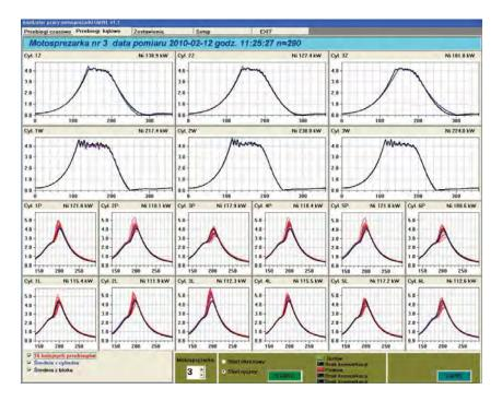
Fig. 5. Main menu of pressure analyzer of GMVH motor compressor monitoring-diagnostic system, presented in on-line mode
