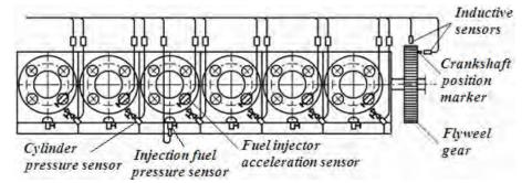
Fig. 2. The scheme of measuring unit of monitoring-diagnostic system used on four bulk carriers to monitor the main propulsion engine Sulzer 6RTA76
