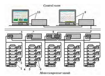
The system covers five motor compressors of GMVH type (Fig. 4).
