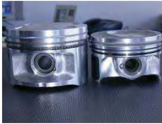
Fig. 1. Comparison of dimensional relation between pistons of modern gasoline engines: piston of 86.4 mm diameter on the left hand side and piston of 76.5 mm diameter on the right hand side
