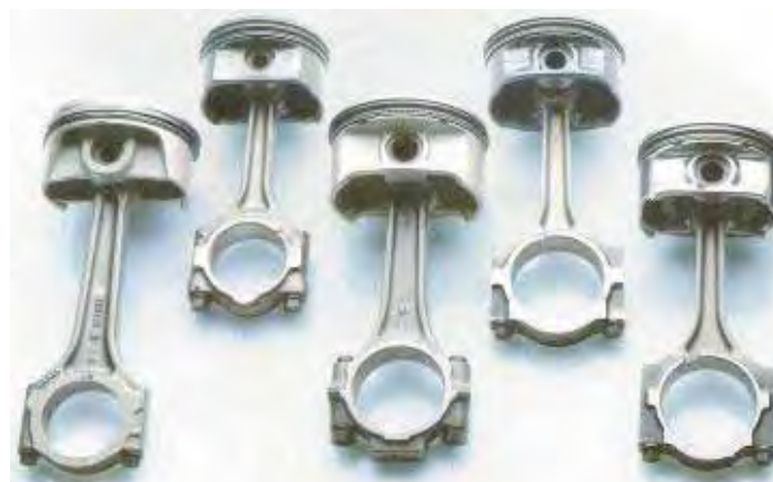
Fig. 3. Comparison of pistons and connecting rods of modern gasoline engines
