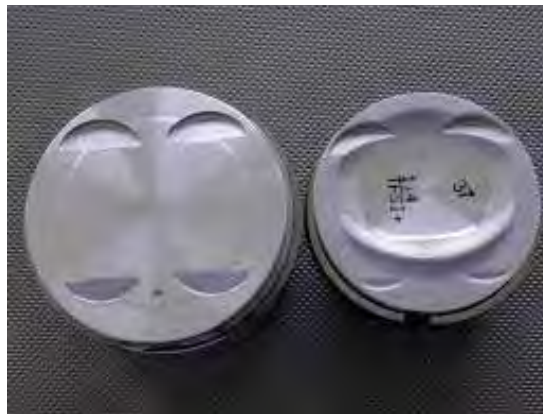
Fig. 2. Comparison of piston crown dimensional relation between pistons of modern gasoline engines: piston of 86.4 mm diameter on the left hand side and piston of 76.5 mm diameter on the right hand side
