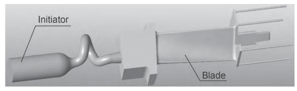
Fig. 1. Model CAD of blade and also initiator
