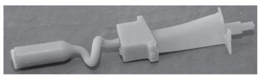
Fig. 5. Model kit from casting wax
