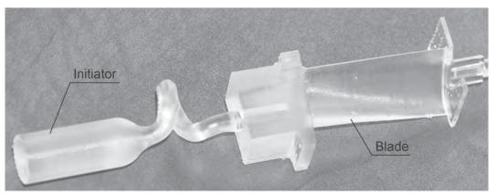
Fig. 3. Model SLA of blade and also initiator
