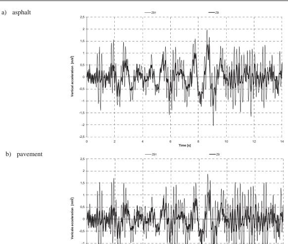
Fig. 7. Vertical accelerations of the vehicle centre of mass (z) and the driver seat (zF) for a vehicle with damaged suspension of one wheel (a – asphalt, b – pavement)
