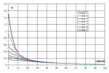
Fig. 4. Dynamic characteristics for a vehicle with reduced engine parameters
