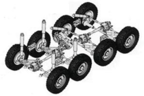
Fig. 2. Drive system scheme
