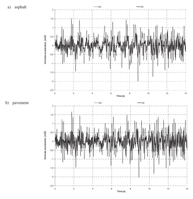
Fig. 9. Courses of vertical acceleration affecting a vehicle with damaged second axle wheels in motion (a - asphalt, b - pavement)
