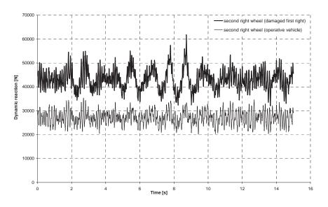
Fig. 8. Dynamic reactions of a selected wheel for operational and damaged vehicles (asphalt)
