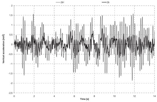
Fig. 6. Vertical accelerations of the vehicle centre of mass – ZB and the driver seat – ZB1 for operational vehicle (asphalt)
