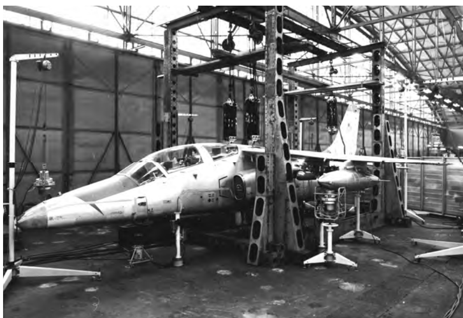
Fig. 3. I-22 Iryda aircraft during the resonance tests
