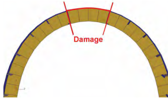
Fig. 4. The initial size of the damage in cross-section (A)
