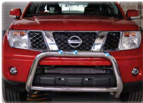
Fig. 1. Frontal protection system fitted to the front of the SUV
