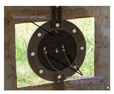
Fig. 10. Experiment station of punching the ballistic shield
