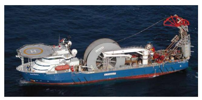
Fig. 1. Pipe laying vessel "Seven Mavica" [www.subsea7.com]
