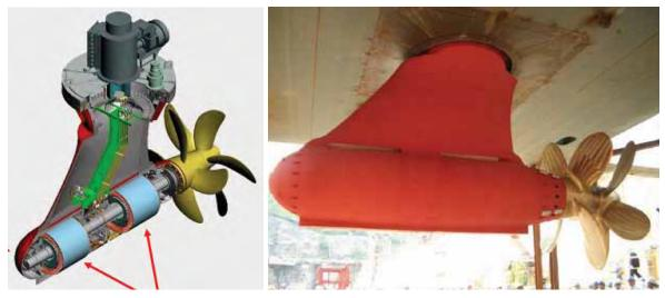
Fig. 3. Contra-rotating pod propellers with two shafts and two electrical motors [5]
