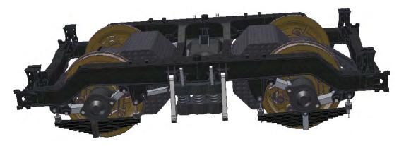
Fig. 2. CAD model of wheel bogie
