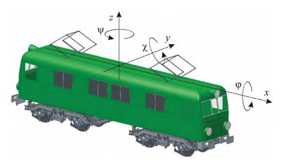
Fig. 1 Model of the vehicle created in Inventor program
