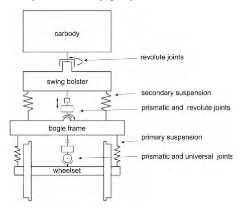
Fig. 3. Physical model of the vehicle under consideration
