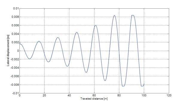
Fig. 6. Lateral displacement of the vehicle wheelsets for a forward velocity of 10 m/s
