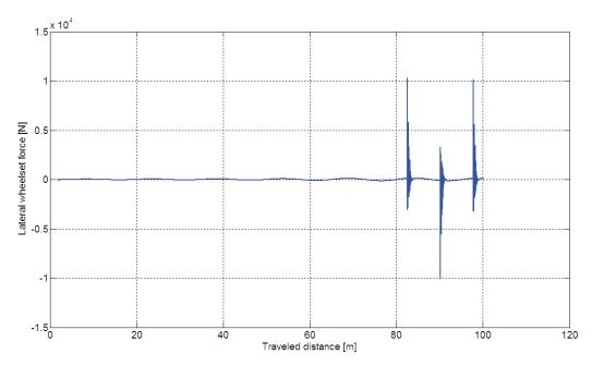
Fig. 7. Lateral contact force on wheelset for a forward velocity of 10 m/s
