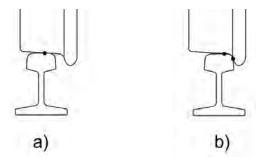
Fig. 8. Different types of contact between wheel and rail: a) tread contact – one point of contact; b) flange contact – two points of contact
